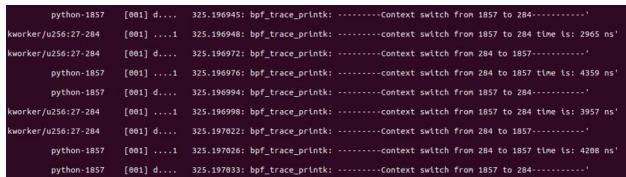
Fig. 6 Test result of process context switch latency 图6 进程上下文切换时延测试结果
